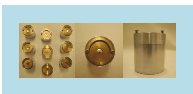
Figure 4 – Schematic side and top views of the effusion cell. a, brass ring; b, brass disk; c, teflon disk; d, platinum foil; e and f, aluminium cell with aluminium lid. At the bottom: picture of the nine cells with a detail of the platinum orifice.
