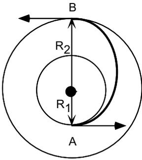
$$\Delta v_A = \sqrt{\frac{GM}{R_1}} \left( \sqrt{\frac{2R_2}{R_1 + R_2}} - 1 \right)$$
