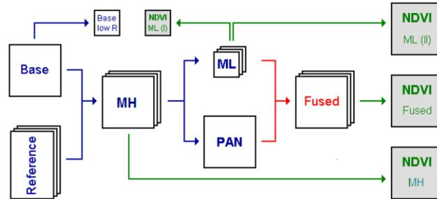
Figure 2. Schematic representation of the data fusion evaluation experiment: MH - multi-spectral high resolution, ML - multi-spectral low resolution and PAN - panchromatic high resolution.
