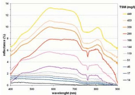
Figure 5. Experimental reflectance profile of water with various levels of TSM concentration.
