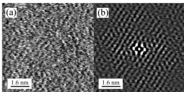
**Figure 4.** AFM image of the SAM of neoglycoconjugate **1** (a) and corresponding autocorrelation function (b).
