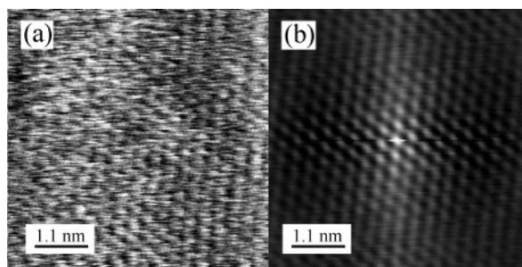
**Figure 2.** AFM constant height mode image (unfiltered) of the gold surface prepared by the TSG method (a) and corresponding autocorrelation function (b).
