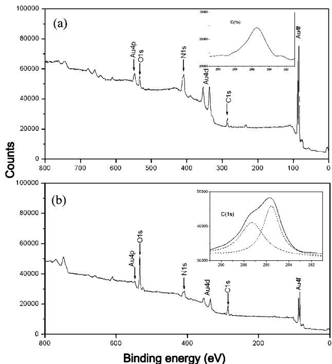
**Figure 3.** XPS survey spectra of respectively gold (a) and the SAM of neoglycoconjugate **1** (b). The insets correspond to a narrow scan in the C(1s) region.
