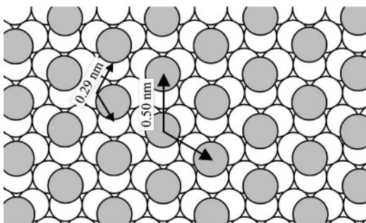
**Figure 5.** Schematic of the  $\sqrt{3} \times \sqrt{3}\text{R}30^\circ$  sulfur superstructure on the (111) gold surface. Filled circles correspond to sulfur atoms.
