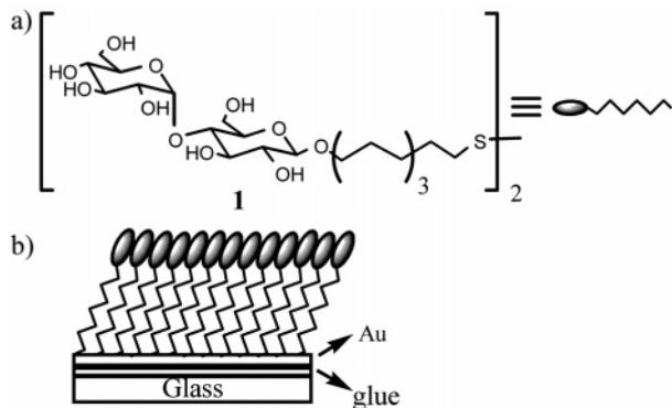
**Figure 1.** Chemical structure of neoglycoconjugate **1** (a) and schematic of the SAM formation (b).
