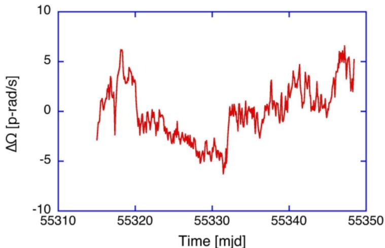
The large ring laser “G” at the Geodetic Observatory in Wettzell has a square contour with an area of  $16 \text{ m}^2$  and a corresponding perimeter of 16 m and is placed on a very stable granite monument in a laboratory approximately 6 m below the Earth surface. A performance level of **better than  $1.26 \times 10^{-11} \text{ rad/s}$  is now routinely obtained.**
