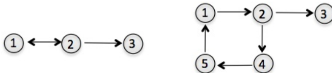
FIGURE 1. The 5-cell network on the right is a lift of the 3-cell network on the left that is not spectrum-preserving.
