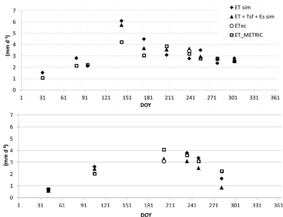
Fig. 4. Evapotranspiration modelled with SIMDualKc ( $ET_{sim}$ ), ET derived from calibrated sap flow data and soil evaporation obtained with SIMDualKc ( $ET = T_{sf} + E_{ssim}$ ), ET obtained with the eddy covariance technique ( $ET_{ec}$ ) and evapotranspiration derived from METRIC ( $ET_{METRIC}$ ) for 2011 (upper panel) and 2012 (lower panel).
