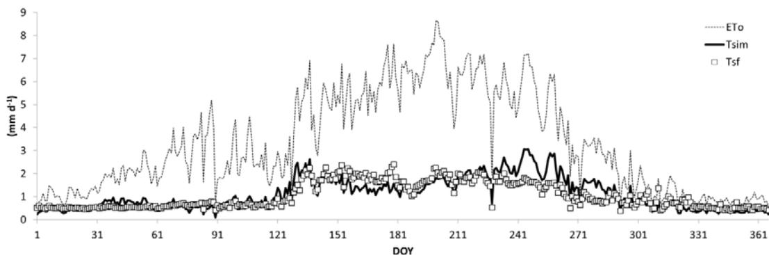
Fig. 3. Plant transpiration modelled with SIMDualKc ( $T_{sim}$ ), calibrated transpiration derived from sap flow data ( $T_{sf}$ ) and grass reference evapotranspiration ( $ET_0$ ) for 2011 (upper panel) and 2012 (lower panel).
