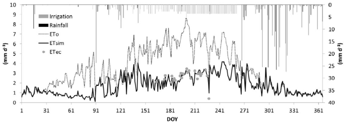
Fig. 2. Evapotranspiration modelled with SIMDualKc ( $ET_{sim}$ ), ET derived from calibrated sap flow data ( $T_{sf}$ ) and soil evaporation obtained with SIMDualKc ( $E_{ssim}$ ), ET obtained with the eddy covariance technique ( $ET_{ec}$ ) and grass reference evapotranspiration ( $ET_0$ ) for 2011 (upper panel) and 2012 (middle and lower panels)
